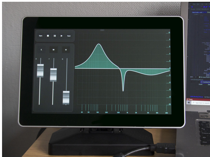
Figure 3.10: The final version of the touchEQ prototype running on the TanvasTouch interface
