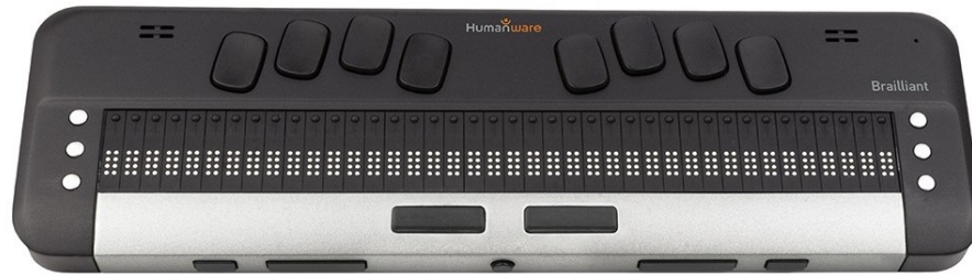
Figure 2.1: A braille display with 40 refreshable cells with a cost of $3,995
